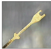
Buckling Beam used for BGA pitches 0.5 mm and below
