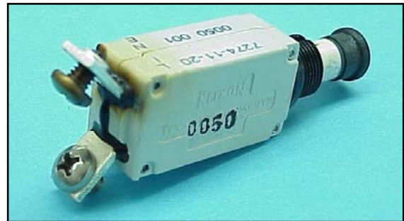
Burned circuit breaker due to external heating from loose terminal screw
