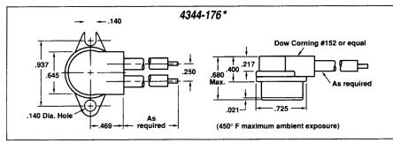
\* An additional ±3°F tolerance is required for overmolded devices.
