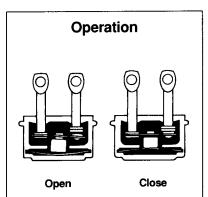
When heated, the internal stresses of the bi-metal cause the disc to reverse its curvature with a snap-action at a fixed, preset temperature and operate the electrical contacts.
